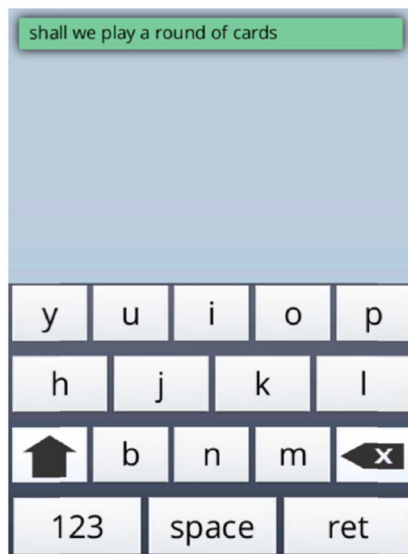
Figure 5. Gesture keyboard, shake the device to see the other half of the keyboard [1]
